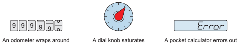
Figure 2.4 Different ways to handle arithmetic overflow. An odometer wraps around from 999999 back to 0; a dial knob simply stops at the maximum possible value; a pocket calculator prints Error and stops.
