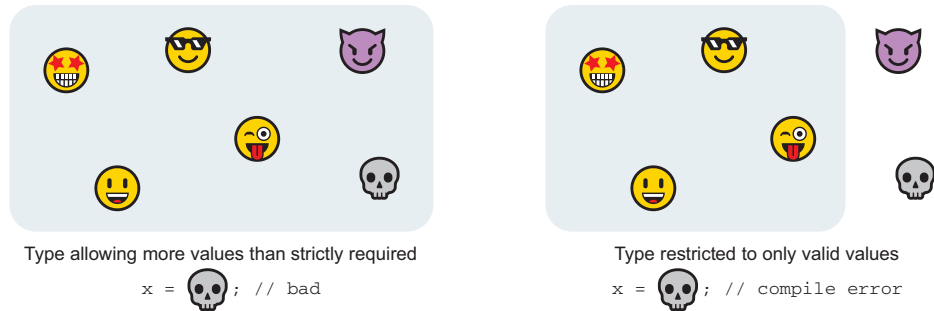
Figure 1.4 Declaring a type correctly, we can disallow invalid values. The first type is too loose and allows for values we don't want. The second, more restrictive type won't compile if the code tries to assign an unwanted value to a variable.
