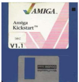
► The original Kickstart came on floppy disk but by the time of the A500 it was a ROM chip on the Amiga motherboard.
