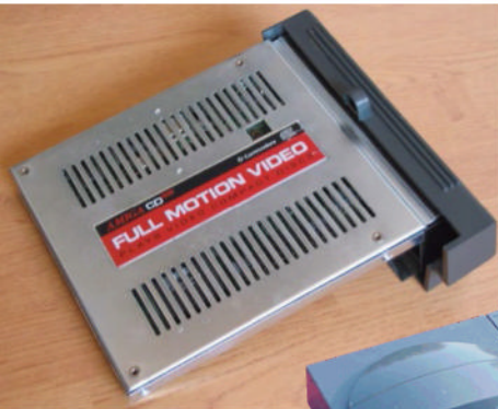
» Above: The FMV Module allowed Video CDs to be played, but was overpriced at £199. Right: Commodore's proposed CD1200 would have allowed the Amiga 1200 to play CD32 games, but was never released.
