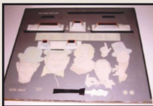
» [Fig. 11] The back of the microprocessor-driven Flicker pinball machine's backglass showing the modifications Jeff and David made to support LED-based scoring (the first of its kind).
