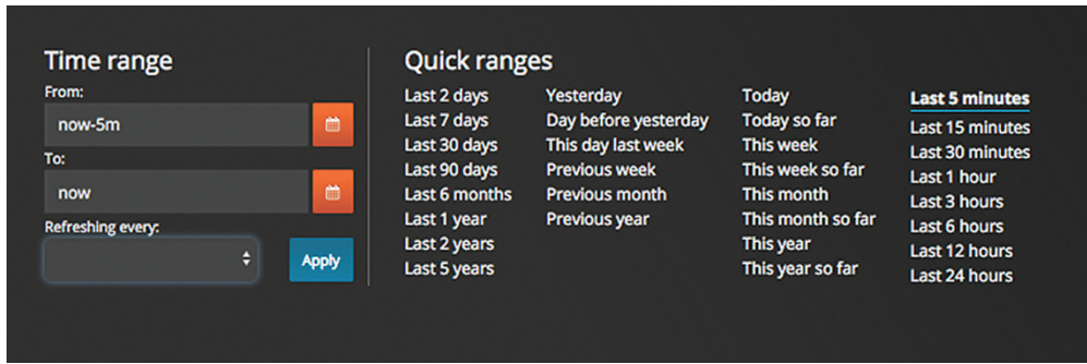
Figure 11.10 Selecting the time range for which you want metrics to be displayed
