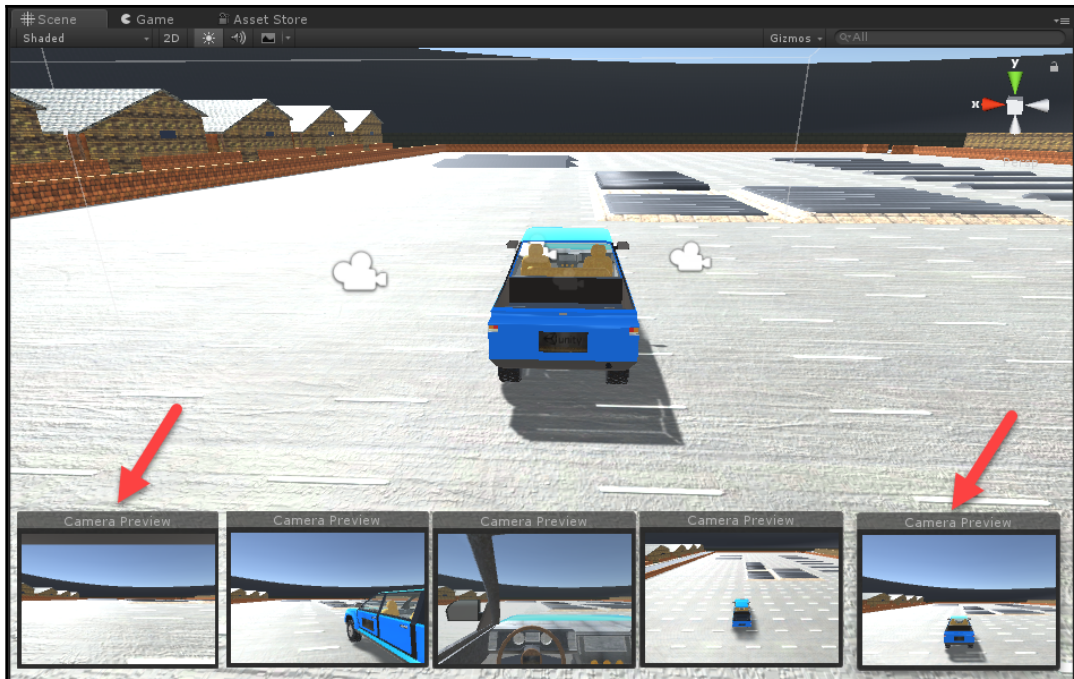
Selecting the visual observation camera to use as an input to the agent
