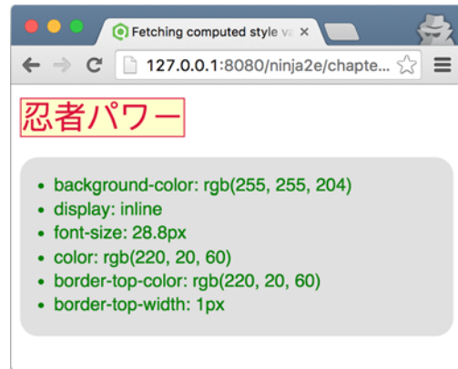
Figure 12.3 Computed styles include all styles specified with the element as well as those inherited from style sheets.
