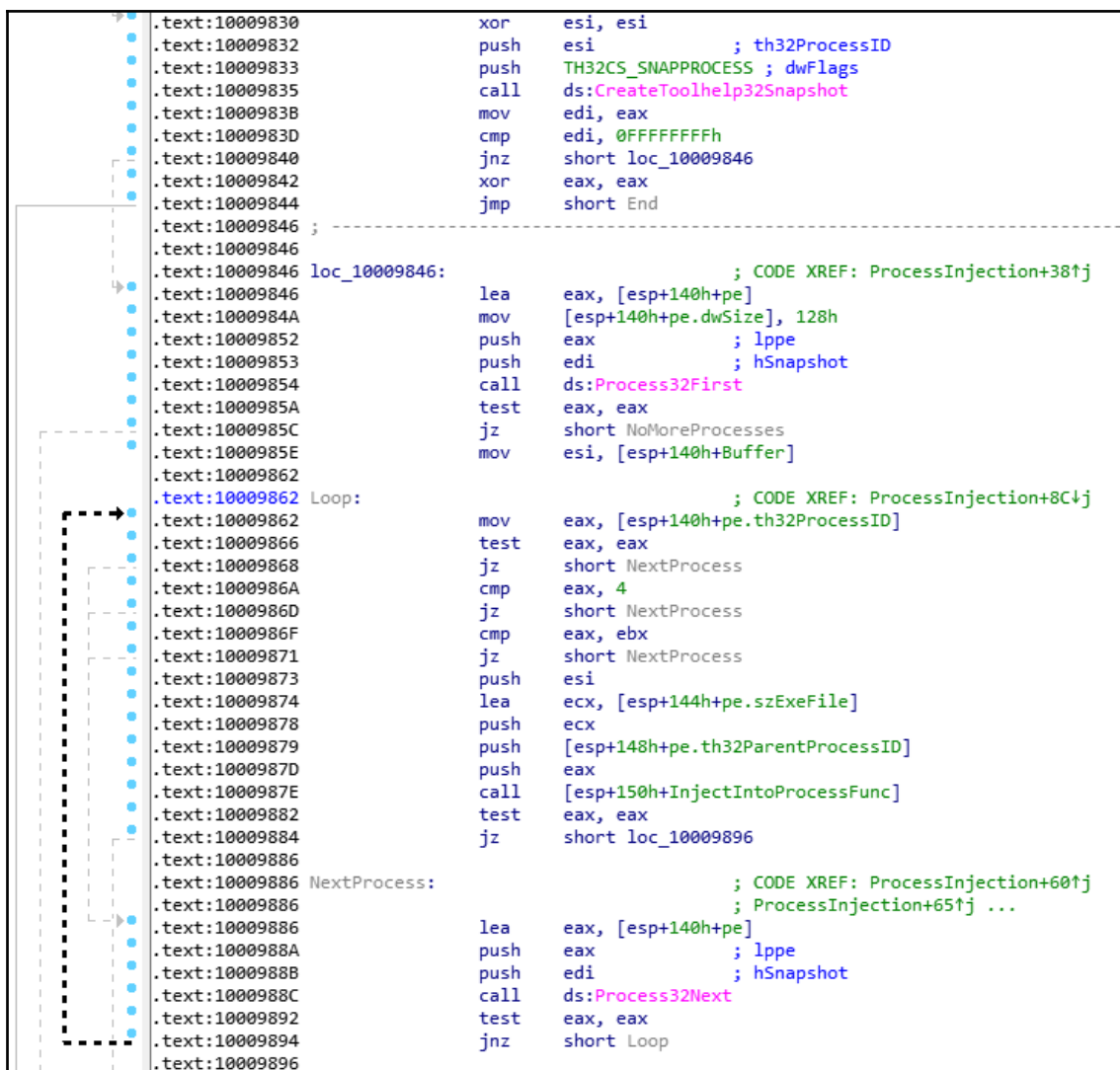
Figure 4: Process searching using CreateToolhelp32Snapshot
