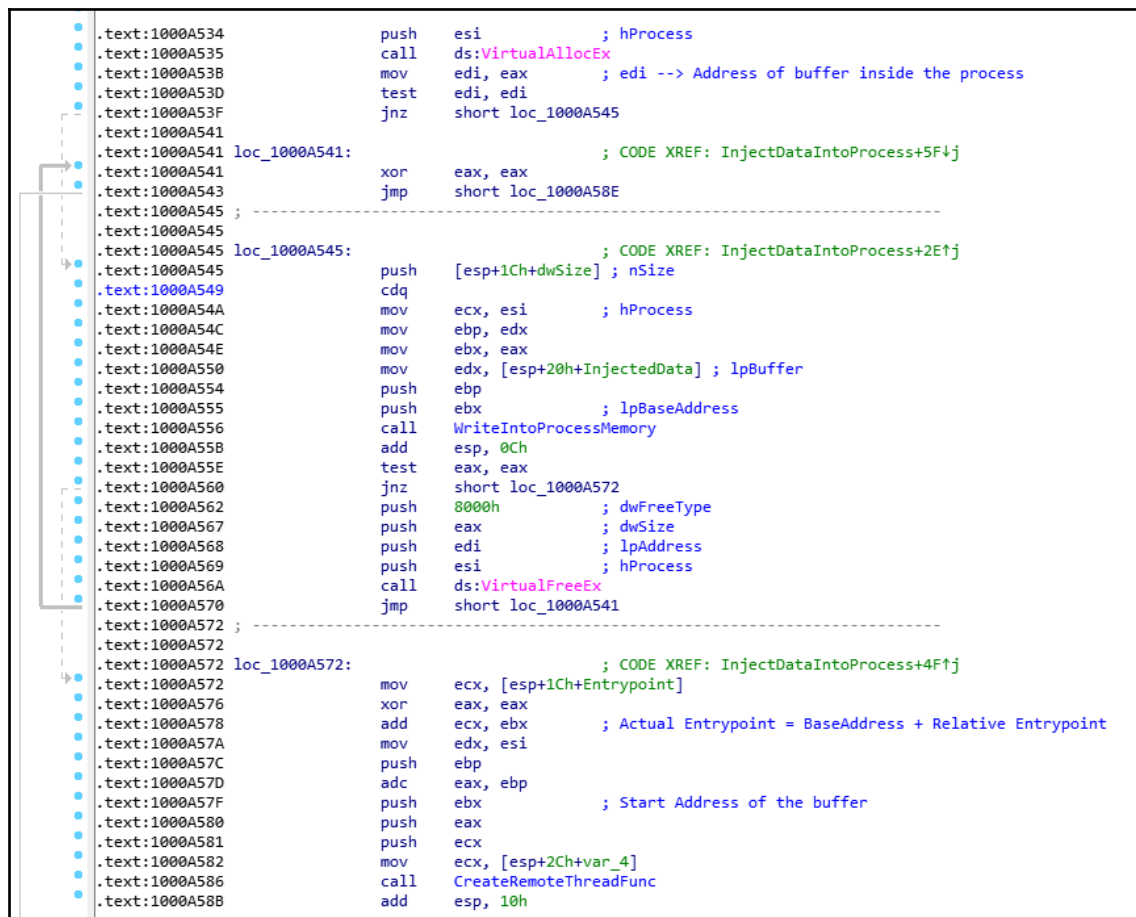
Figure 5: Code injection example
